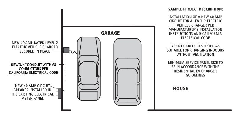
Though an individual Level 2 EV charger may have a negligible impact on the utility electric system, the combined effect of several chargers in the same neighborhood could result in overloads on utility secondary wires and transformers. It is important that the local PG&E office be notified of any Level 2 charger installations to ensure that utility electrical system components are adequately sized to maintain high levels of service reliability.
