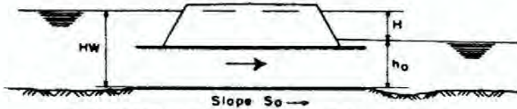
SUBMERGED OUTLET CULVERT FLOWING FULL
