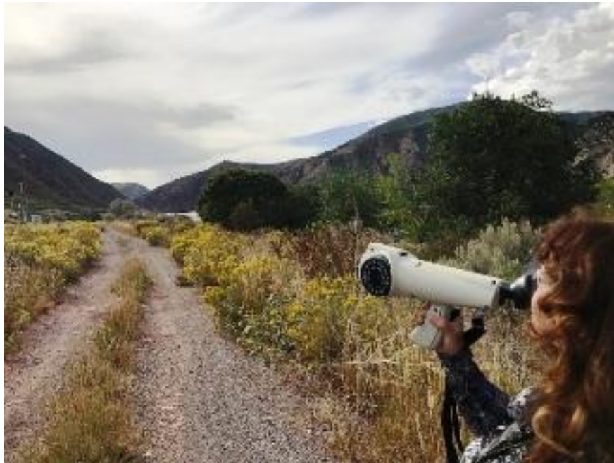
Figure No. 1 – Nasal Ranger Olfactometer
