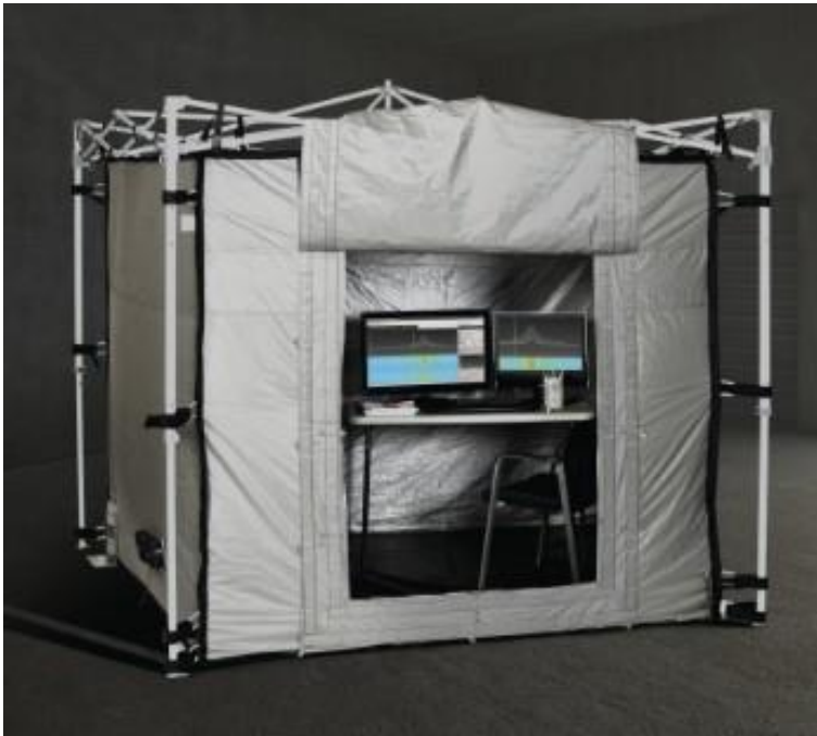
Image – An example of a Faraday tent shielding a desktop system. Source: Faradaydefense.com
