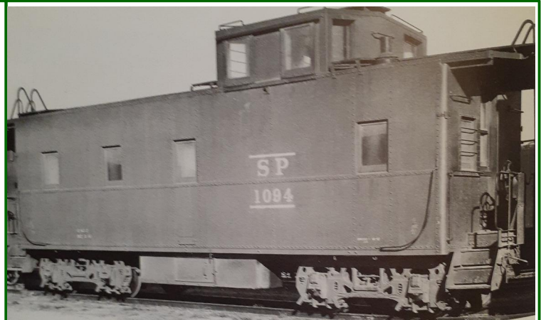
(Top) SP 1094 still had its Allied trucks and original paint at Bayshore in 1947. Although Southern Pacific found the ride quality of Allied trucks fully satisfactory, they were a source of maintenance problems, as was true on other railroads which used them. All the Allied trucks on SP cabooses would be replaced with Vulcan or Barber-Bettendorf trucks between May, 1949 and July, 1950. (E.R. Mohr photo, Paul Koehler collection)
