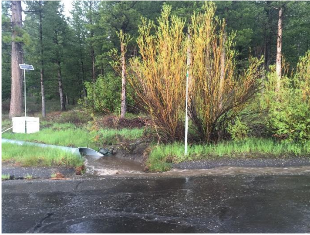
Figure S7. Sampling stations installed on Elks Club Drive for stormwater runoff collection before (year 1, left) and after (year 2, right) pavement rehabilitation.
