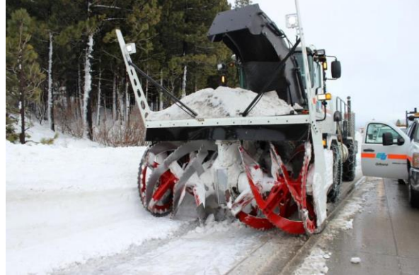
Figure S3. Snow plow equipped with a metal blade (left) and rotary blades mounted on a snow blower (right), operated by El Dorado County to remove snow from roads.
