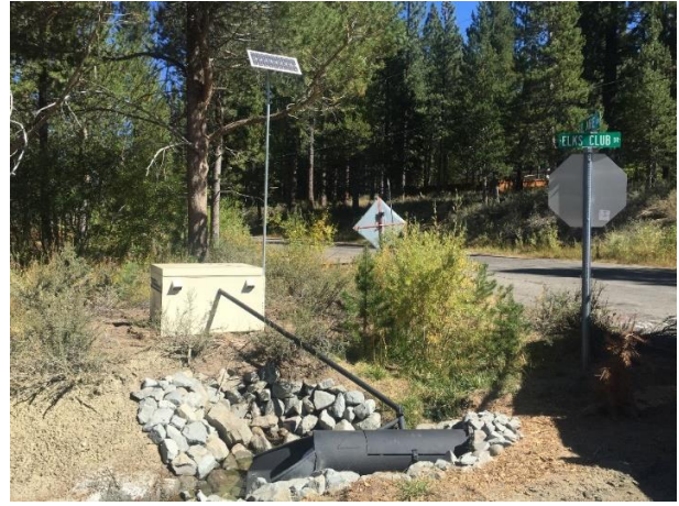
Figure S7. Sampling stations installed on Elks Club Drive for stormwater runoff collection before (year 1, left) and after (year 2, right) pavement rehabilitation.
