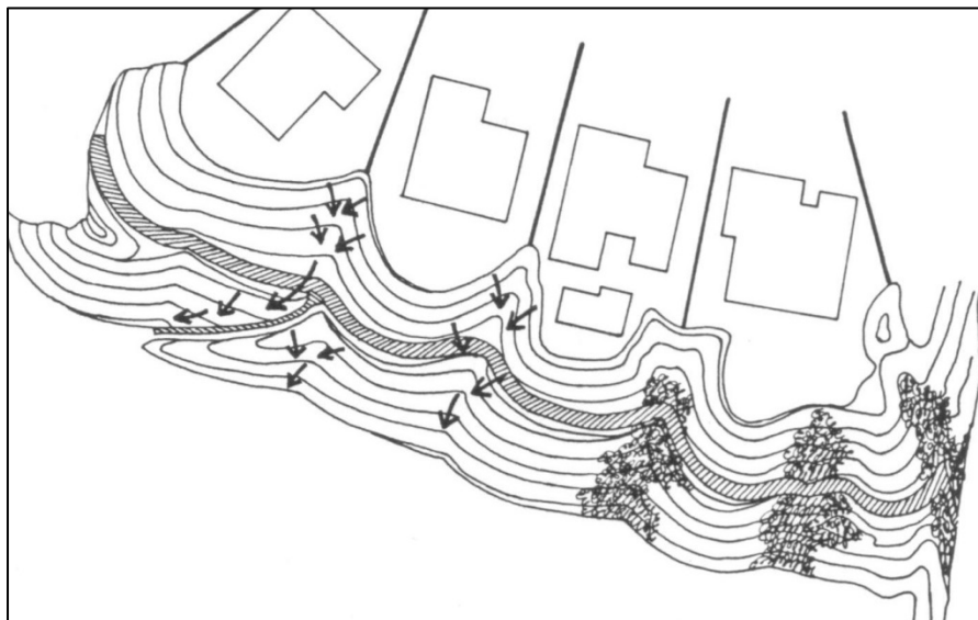
Figure B.6 – Contour Grading Example
