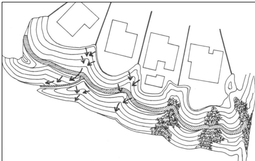
Figure B.6 – Contour Grading Example
