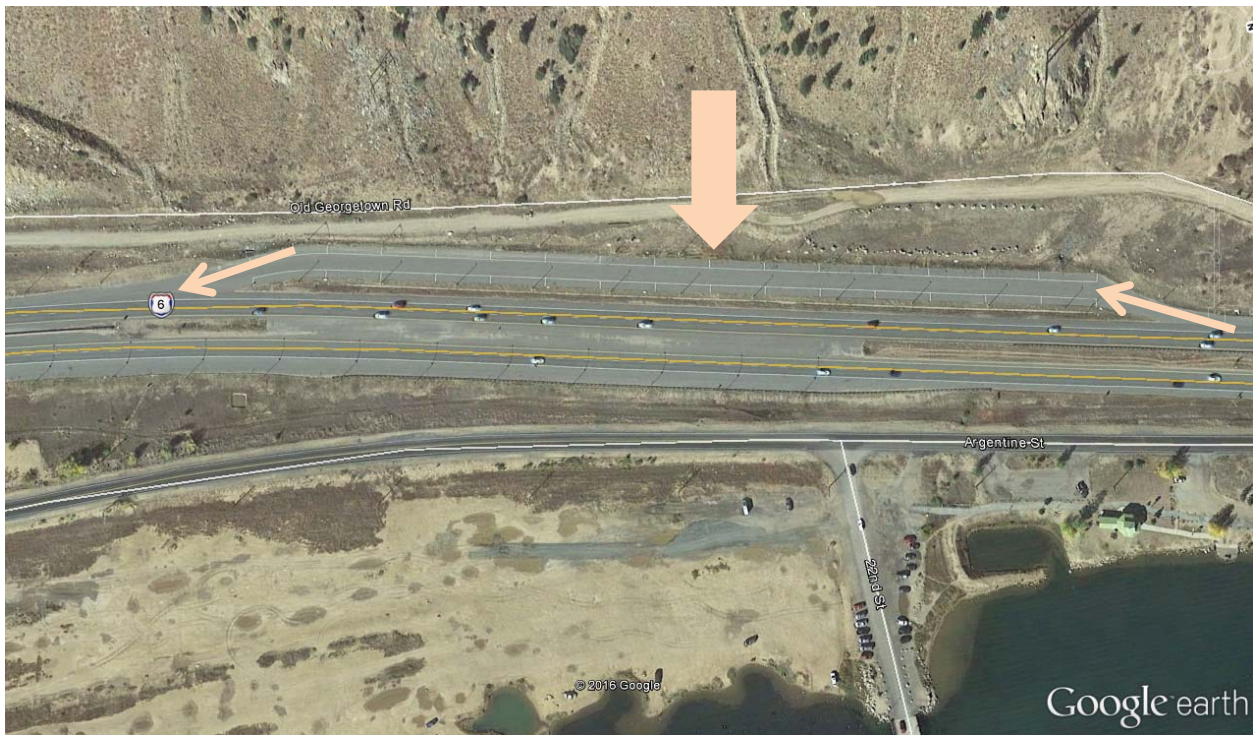
Figure 19: Separate Chain Up Example from I-70 in Idaho Springs, CO 24 and Georgetown, CO 25 (Aerial Image Source: Google Earth)
