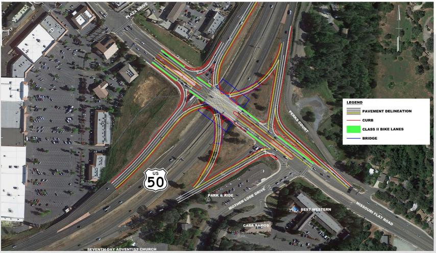
Combines 2 ramp intersections into a single intersection on bridge.
