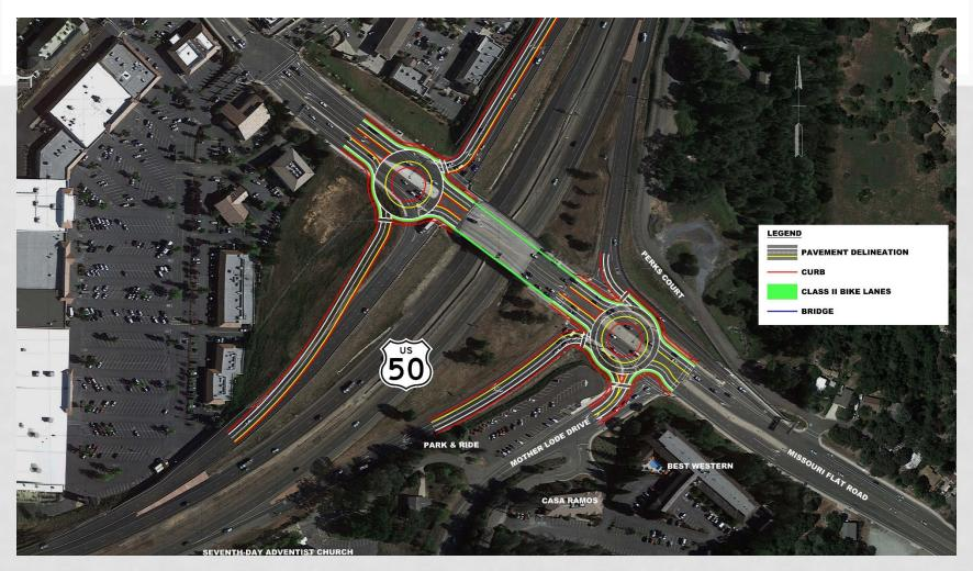
Provides roundabouts at ramp intersections
