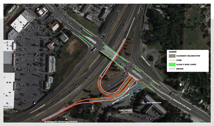
Provides new EB On/off-ramps connecting to Missouri Flat Road in standard configuration. (Requires Motherlode Drive Relocation)
