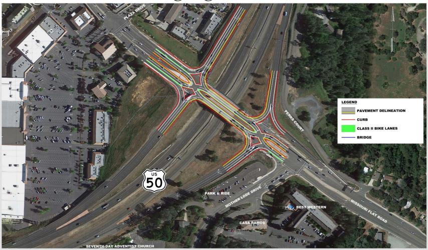
Switches traffic on bridge to left side to allow more efficient traffic operations
