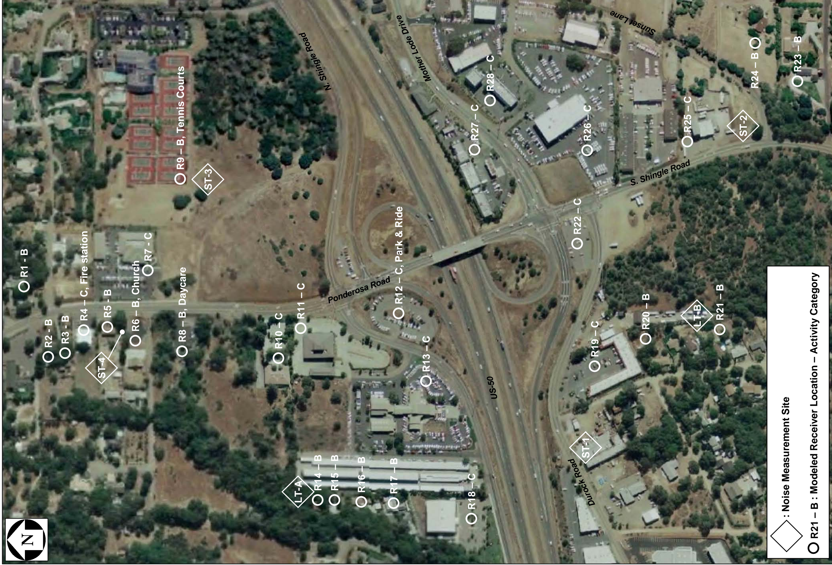
Figure 13 US-50 / Ponderosa Road Interchange Noise Study Noise Measurement Sites and Modeled Noise Receptors
